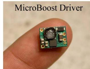
Warning: This driver is a current source mode driver. Do not disconnect the laser diode while operating, diode damage may result. Use secure solder joints for laser diode connection.
